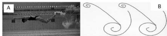
Figure 4. An exemplary image of the vortices generated during underwater undulatory swimming with the injecting bubble visualisation technique (A) and a sketch of the generated vortices of the wake (B) (alteration from Arellano, 1999).
