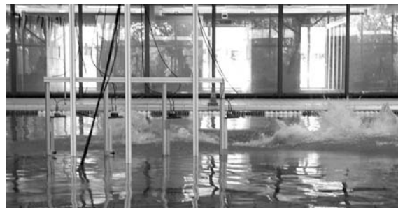
Figure 3. Left panel: The four wave probes, registering wave amplitude, were located at a fixed distance from the MAD-system. The distance between the wave probes was 0.5 meter; the probes covered half a stroke-cycle of the swimmer. For each probe the wave resistance was calculated. It seemed that the wave resistance varies during the stroke.
