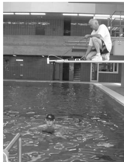
Figure 1. Measuring procedure using the Doppler-Ultrasound-Velocimeter System.
