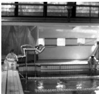
Figure 1. Image of recording a swimmer's impulse on the force platform by the high speed camera. In gray lines, segment's modelling using passive markers.
